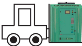
RIGHT WAY Forklift forks need to overtake the equipment.
