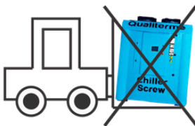
WRONG WAY Forklift forks need to go beyond all equipment to avoid damage to components.
